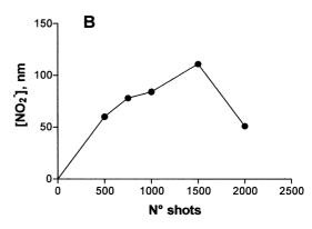
Fig. 2. Production of nitrites in the the presence of 10 mM L-arginine and 1 mM  $\rm H_2O_2$  at constant number (1000) of shots of increasing energy levels of SW (A), and at constant energy (0.89 mJ/mm²) of increasing number of shots (B). The experiments were performed using three identical samples for each condition tested (triplicate measurements/sample). Standard deviations were comprised in the range of 8.5-19.4%, for all values.
